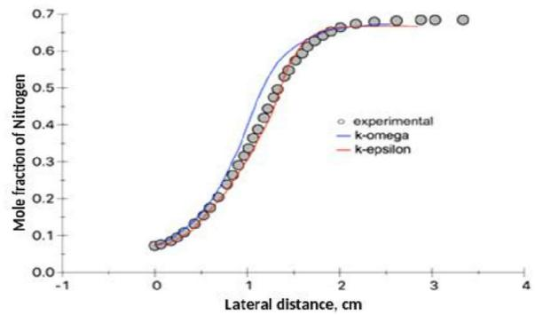
FIGURE 5: COMAPARISON OF N<sub>2</sub> EXIT PROFILES
