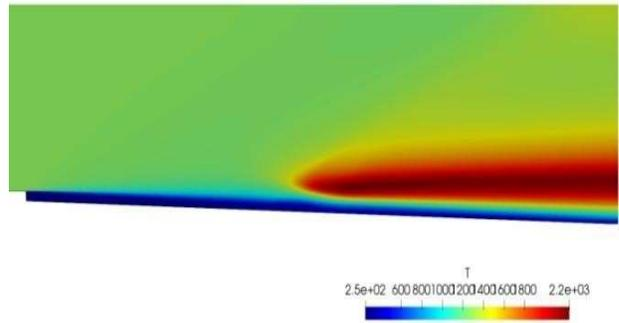
**FIGURE 11:** TEMP. CONTOUR OF REACTING CASE (7 STEP CHEM.)
