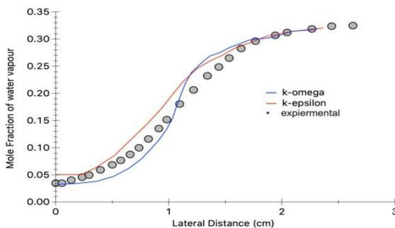
FIGURE 4: COMPARISON OF H<sub>2</sub>O EXIT PROFILES WITH DIFFERENT TURBULENCE MODELS
