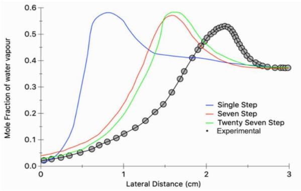
**FIGURE 7:** COMPARISON OF WATER MOLE FRACTION AT EXIT WITH DIFFERENT CHEMISTRIES.
