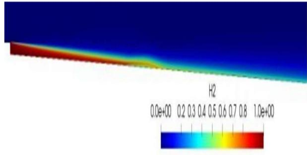
**FIGURE 12:** H<sub>2</sub> CONTOUR OF REACTING CASE (27STEP CHEM.)
