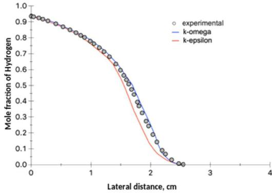
**FIGURE 8:** COMPARISON OF H<sub>2</sub> MOLE FRACTION.
