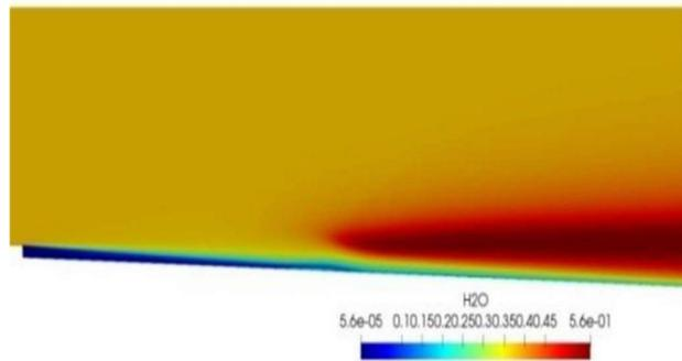
**FIGURE 13:** H<sub>2</sub>O CONTOUR OF REACTING CASE (27 STEP CHEM.)
