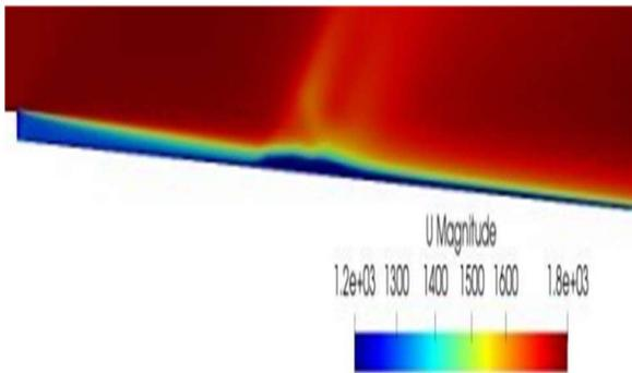
**FIGURE 17:** VELOCITY CONTOUR (27 STEP CHEM)
