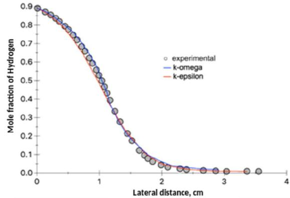
FIGURE 6: COMPARISON OF H<sub>2</sub> EXIT PROFILES
