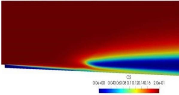
**FIGURE 15:** O2 CONTOUR OF REACTING CASE (27 STEP CHEM)
